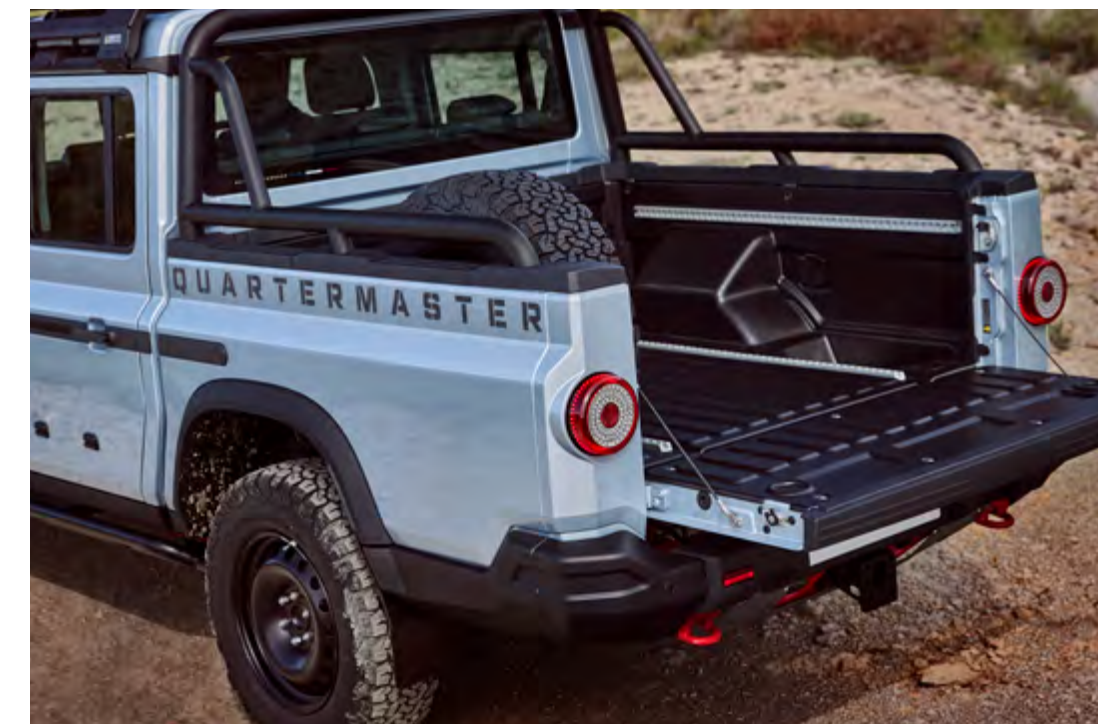
Longer wheelbase results in a load bay that can carry a standard Euro pallet
